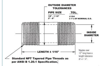
Steel Barrel Nipples with ASTM A733 Standard
